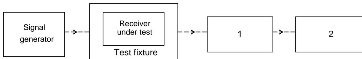
NOTE 1: Coupling device, e.g. AF load/acoustic coupler (in the case of speech equipment).
