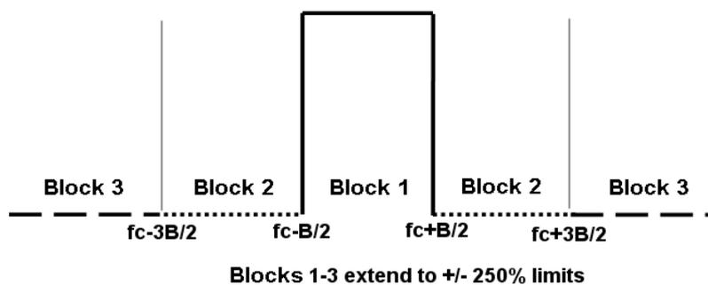
**Figure 1: Measurement Mask normalized to channel bandwidth**
